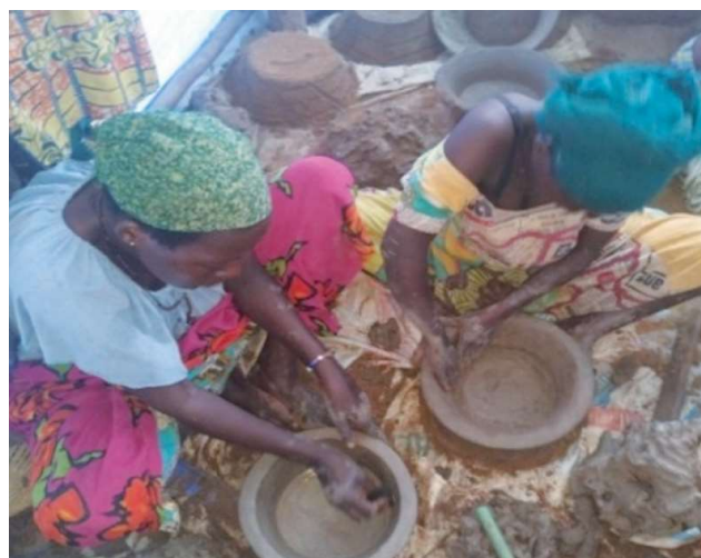
Manufacturing of energy conserving furnaces/ stoves and local employment
